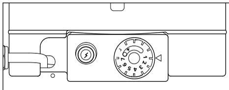
For an higher availability of hot water, it is advisable to leave the knob to position (5) and to mix the water to get the desired temperature.
